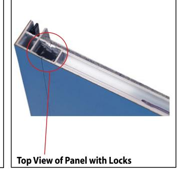
The first level of components contains panel locks that are located at the top of the panel for extra stability and a seamless connection. When disassembling panels, twist top connection slightly and lift right panel upward.
