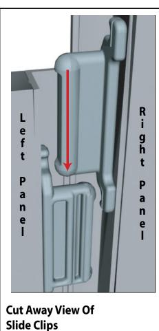
Components connect together by aligning them and sliding downward connecting clips together.
